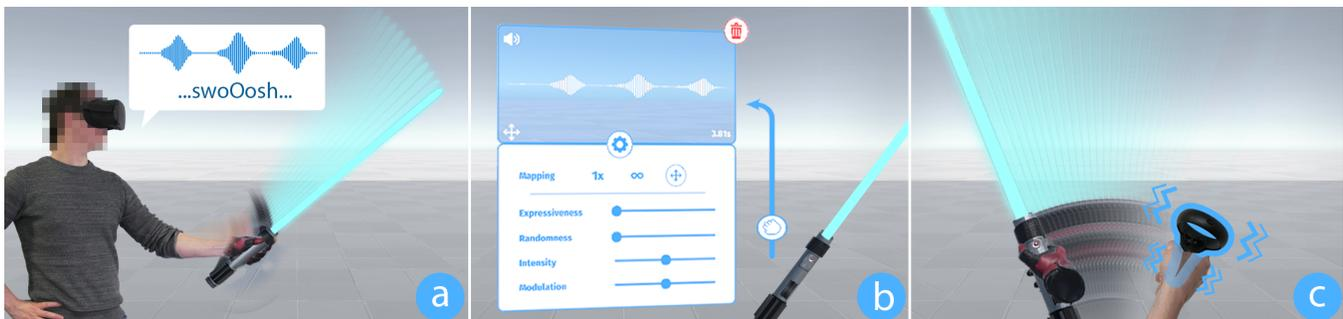
**Figure 1:** With the Weirding Haptics design tool, one can design vibrotactile feedback in a virtual environment using their voice. a) A designer waves a lightsaber in the air while vocalizing the intended feedback. b) A *vocalization layer* depicts properties of the tactile experience and allows for switching mappings as well as fine-tuning using modifiers (sliders) directly in VR. c) While waving the lightsaber, the vibrotactile feedback can be felt with the VR controller.
